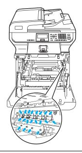
Hold the handles of drum unit when you carry it. DO NOT hold the sides of the drum unit.
